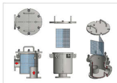
MUD BOX (STEEL PLATE)
